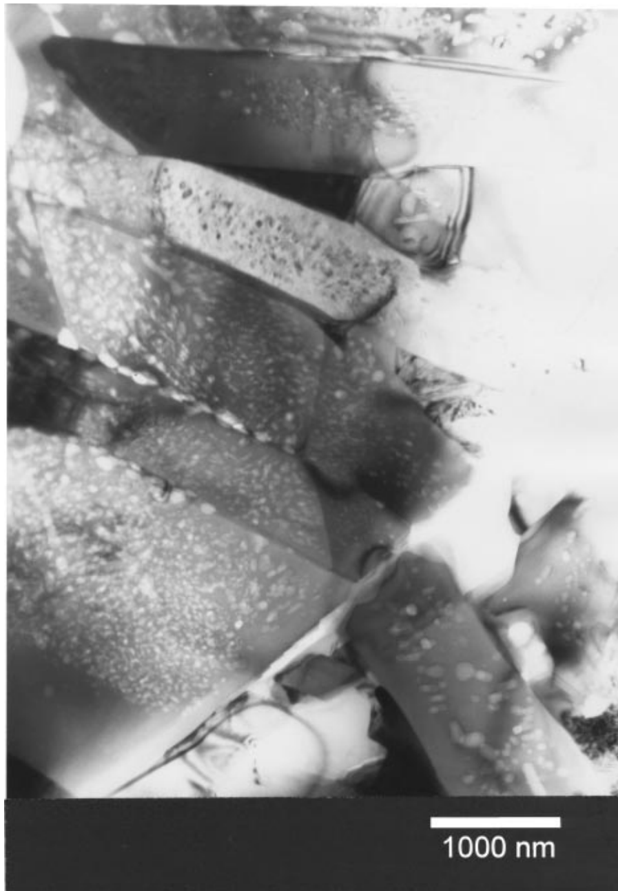
Figure 6 TEM micrograph of a splat in material heat treated at 1180°C, showing lath-like grains after transformation to \alpha -Al 2 O 3 and increased intra-splat porosity.
